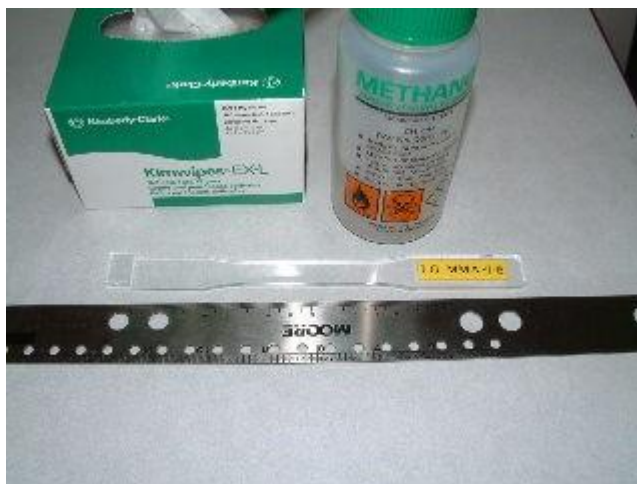
Sample (Piece cut to fit prism on left), Methanol, and Laboratory Tissues
